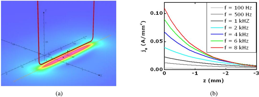
**Fig. 1.** (a) Illustration of FEM-simulated eddy current distribution at the surface excited by one wire. (b) Eddy currents  $j_0$  as function of the depth  $z$  beneath the wire for different excitation frequencies.
