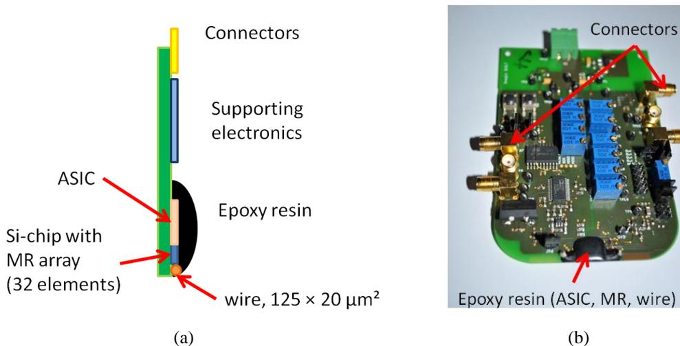
**Fig. 2.** (a) Scheme of the PCB (not to scale) with excitation wire, MR array (GMR or TMR), and ASIC protected by an epoxy resin. In addition supporting electronics and connectors are placed on the PCB. (b) Photo of the IMAGIC TMR probe.
