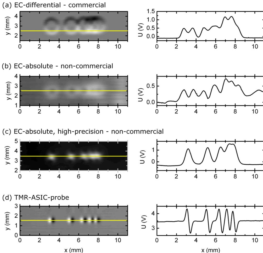
**Fig. 5.** ET-data of Aluminum-sample Al-FN-22 for different probes ((a) differential probe “KDS 2-2” of *Rohmann GmbH*, (b) absolute probe BAM-made “A05”, (c) absolute, high-precision probe BAM-made “AN05”, and (d) TMR-ASIC-probe of the IMAGIC consortium for surface breaking defects) as grey-scaled plots on the left and as line cut across defect signals on the right.
