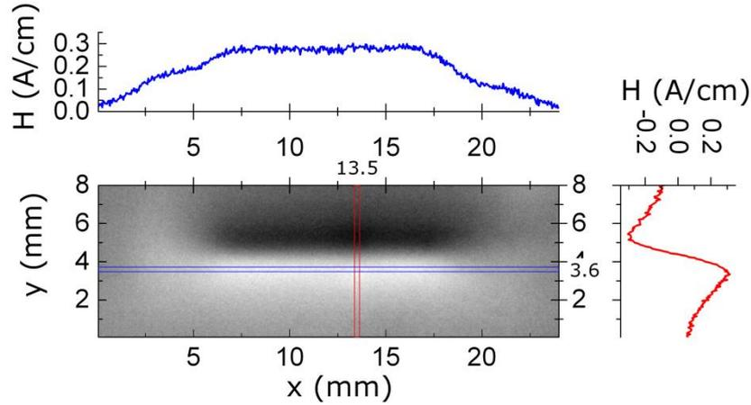
**Fig. 3.** Grey-scaled representation of the magnetic field distribution excited by a wire of a MR surface probe for an excitation current of  $I = 400$  mA. The field strength was measured using a Hall-sensor. Line strips of the field distribution parallel (blue stripe and curve) and perpendicular (red stripe and curve) to the wire. The maximum and minimum magnetic field excited by the wire in a distance of  $500 \mu\text{m}$  is  $\pm 0.35$  A/cm.
