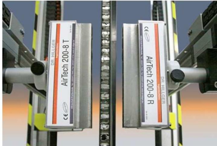
**Figure 3.** AirTech transmitter and receiver arrays
