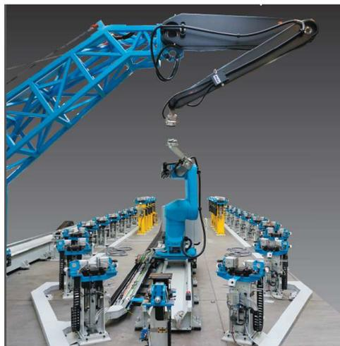
**Figure 6.** Air-coupled ANDI system with two robots [13]
