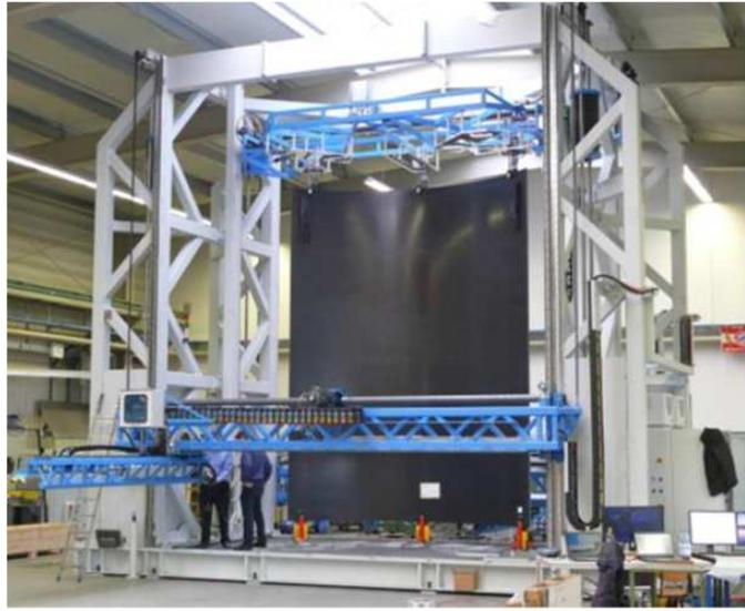
**Figure 5.** 10-axes-scanning system for non-contact inspection of sandwich space-structures
