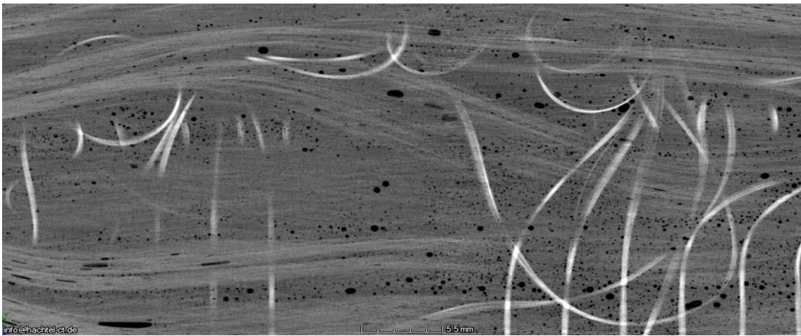
Fig. 5. Ondulation of carbon fibres (light grey) and glass fibres (white)
