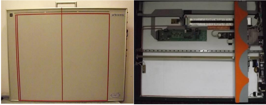
Figure 10 .The dual-energy Flat Panel detector developed
