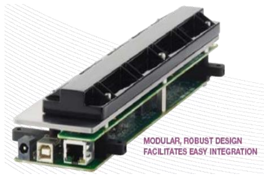
Figure 1. The TDI detector used in our TDI-based Flat Panel detector
