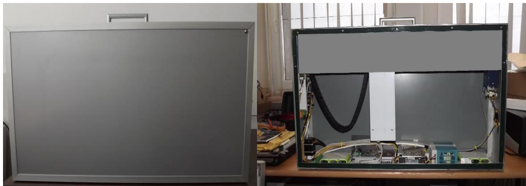
Figure 2. The Flat-Panel detector developed based on TDI detector
