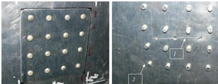
Pic.11. The doubler front and back views. Primer (1) and secondary (2) fatigue cracks
