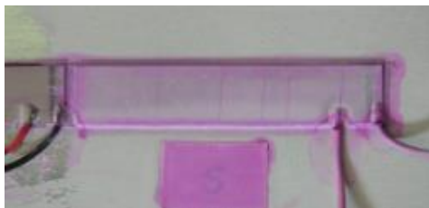
Pic.1. Crack of the PZT after 60000 cycles of fatigue test
