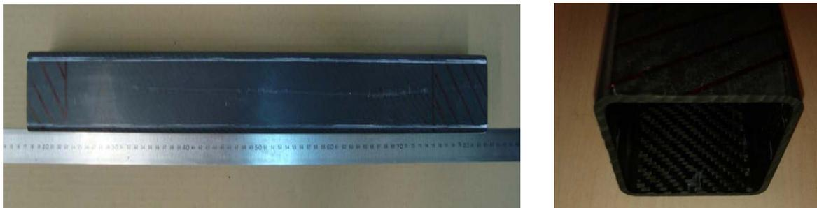
**Fig. 1.** Images of a CFRP specimen for the study of delamination produced by impact.
