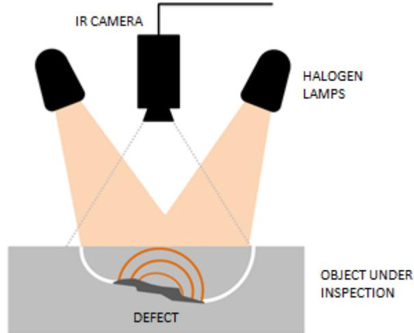
**Fig. 3.** Illustrative scheme of the lay out of the active IRT inspection conducted in the study.
