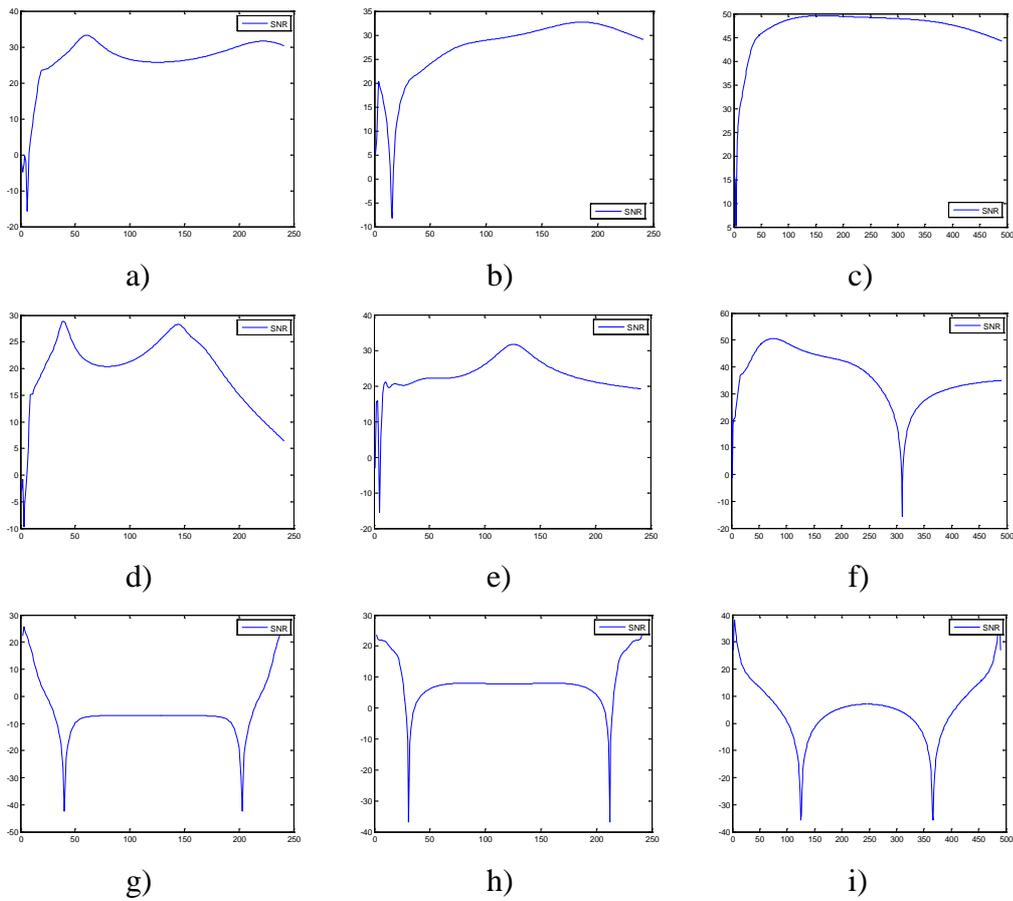
**Fig. 4.** Examples of graphical representation of the behaviour showed by defects under different processing algorithms. First derivative of tsr: a) delamination, b) porosity and c) debonding. Second derivative of tsr: d) delamination, e) porosity and f) debonding. Phase of FFT: g) delamination, h) porosity and i) debonding
