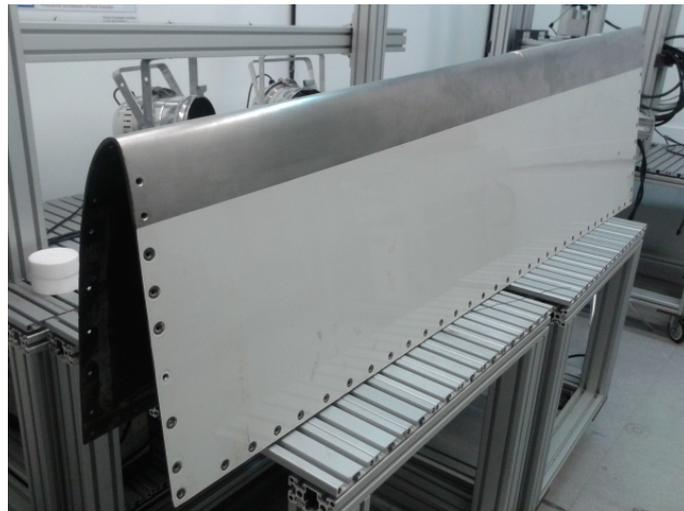
**Fig. 2.** Image of the component containing defects of debonding between CFRP and Ti plate.
