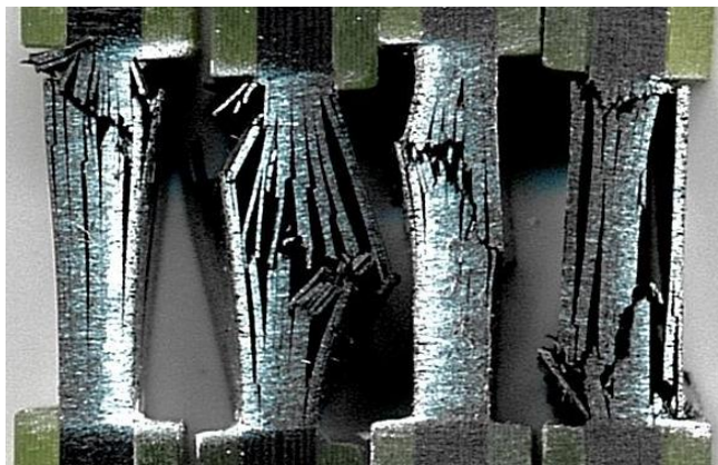
Figure 19: Example of four successfully tested specimens with acceptable failure modes and areas according to ASTM 6641
