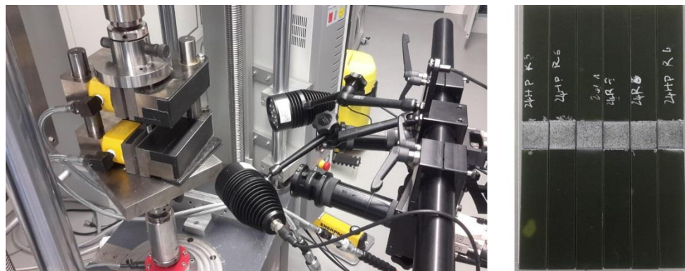
Figure 9: Compressive loading setup and Aramis 12M measuring system (left);
