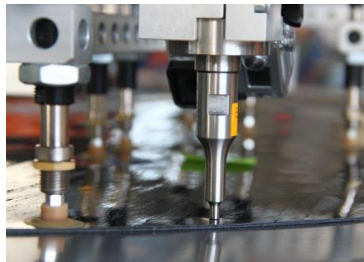
Figure 2: Ultrasonic horn integrated in an end effector for the spot welding of laminate stacks
