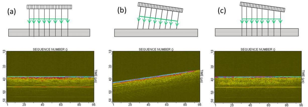
**Figure 6.** (a) Bscan images in a composite plate with 6.5 mm thickness: image when the probe is parallel to the surface (a); images when the probe is inclined of  $5^\circ$  without adaptive processing (b) and by applying SAUL with 2 iterations.
