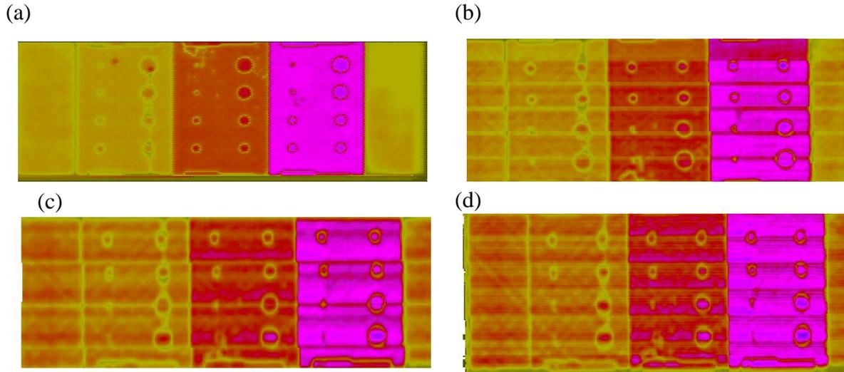
**Figure 2.** CScan images of the artificial defects with different diameters and distributed over three different thicknesses (from right to left 3.5mm; 6.5mm and 10mm): (a) Single-element control; (b) Focused electronic scanning; (c) Optimized S.P.W.T; (d) Classical S.P.W.T
