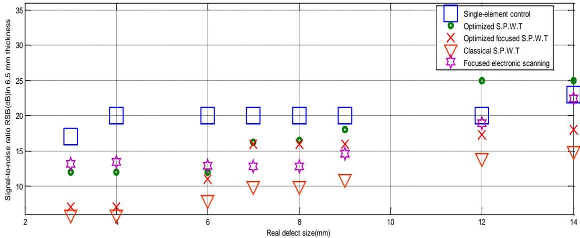
**Figure 3.** Evolution of the SNR for the 6.5-mm thickness part according to the defect size.
