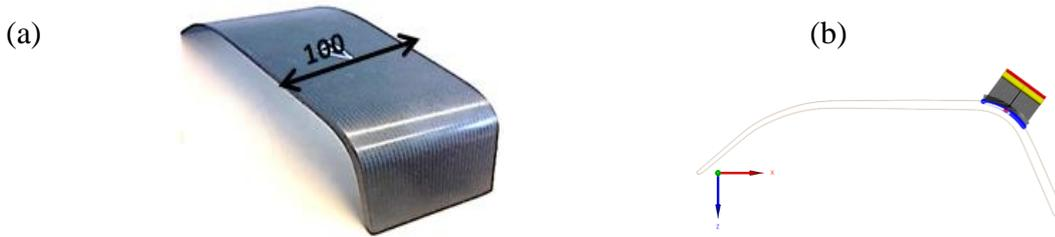
**Figure 7.** Foot prosthesis with a complex geometry ; (a) Perspective view of the foot plate; (b) profile view of the transducer and the foot plate
