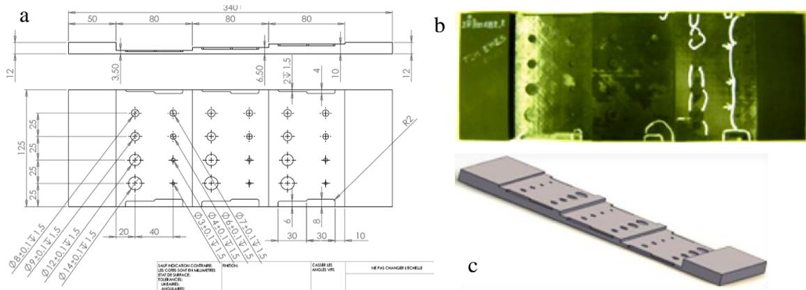
**Figure 1.** The aerospace standard made of carbon epoxy composite and including artificial defects: (a) Drawing definition; (b) Top view; (c) 3D view.
