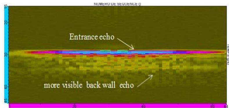
**Figure 10.** Application of the adaptive technique with a 1.5MHz probe.
