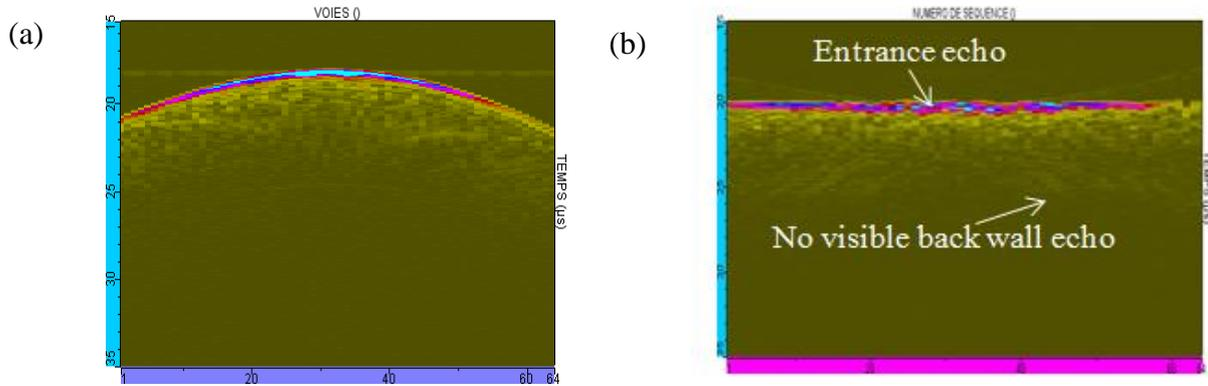
**Figure 9.** Application of the adaptive technique SAUL: (a) BScan (channels/time) before the application of SAUL technique; (b) BScan (channels/time) after application of the SAUL technique.
