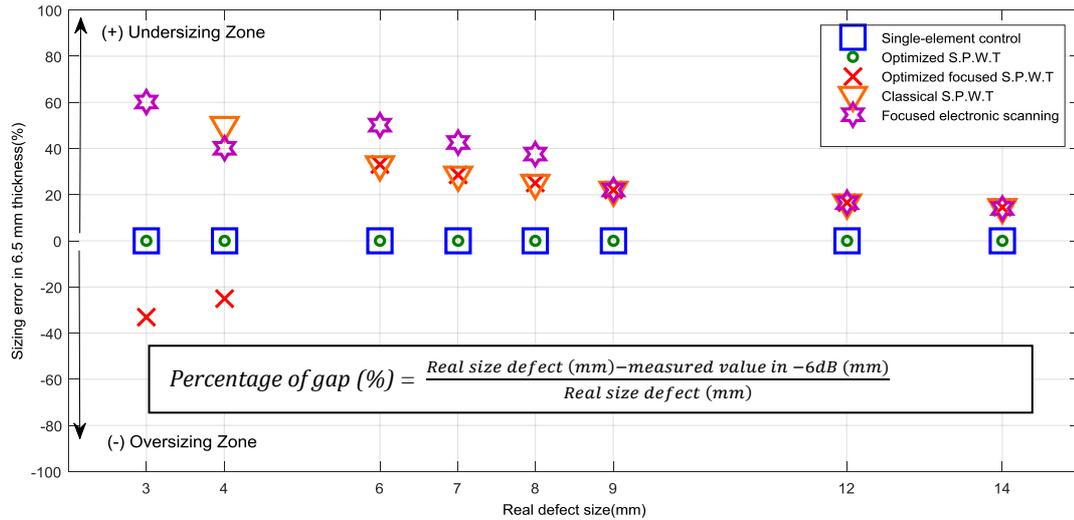
**Figure 4.** Evolution of the sizing error (%) for the 6.5-mm thickness part according to the defect size.
