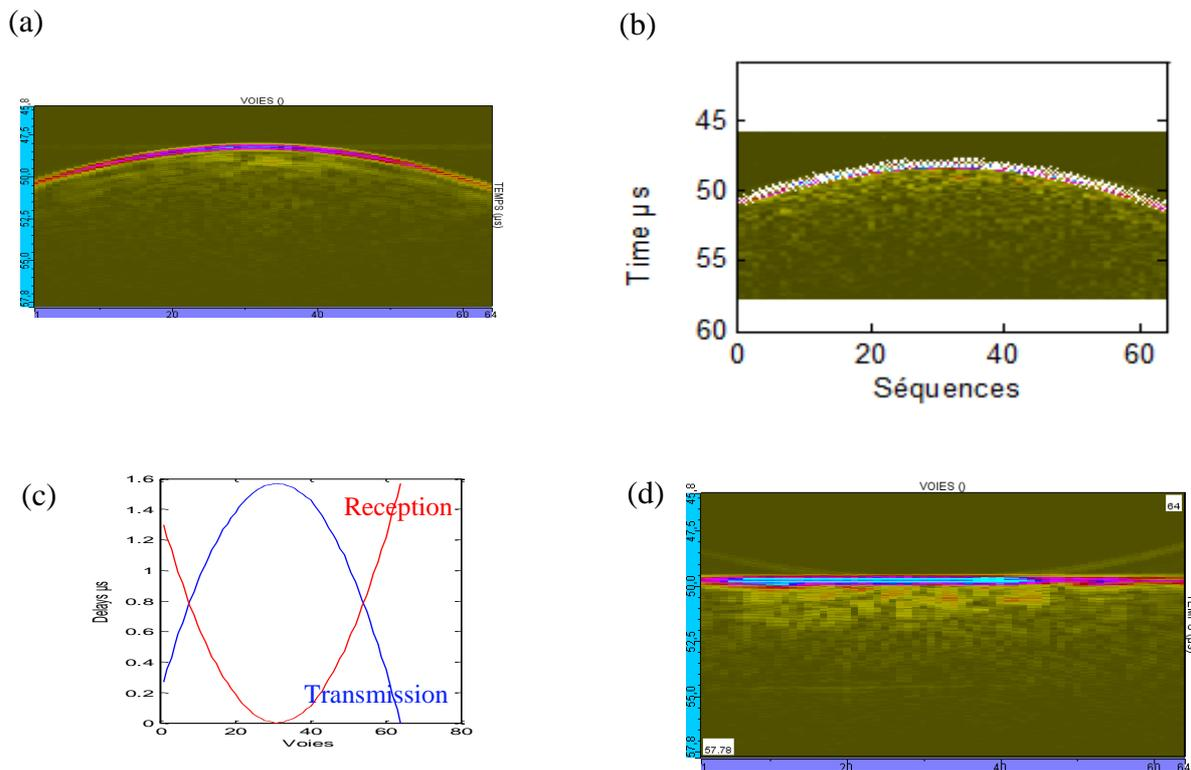
**Figure 8.** Illustration of adaptive linear scanning with a fixed position of the transducer in the center of the convex portion: (a) Bscan image obtained from an electronic scanning in transmission; (b) The time of flight curve superposed to the Bscan image obtained from an electronic scanning in transmission; (c) Delays laws deduced from an electronic scanning in transmission; (d) Bscan image obtained when adaptive delay laws are deduced from an electronic scanning in transmission.
