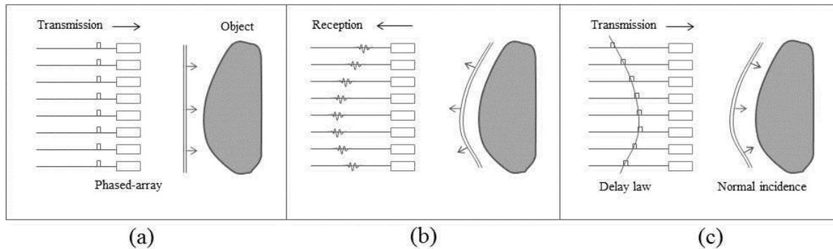
**Figure 5.** Three steps of first SAUL iteration: a plane wave is transmitted by firing with the full array (a); the reflected wave is received by the array and times of flight are measured (b); a delay law is deduced from these measurements and applied to obtain an incident wave-front parallel to the object surface (c).
