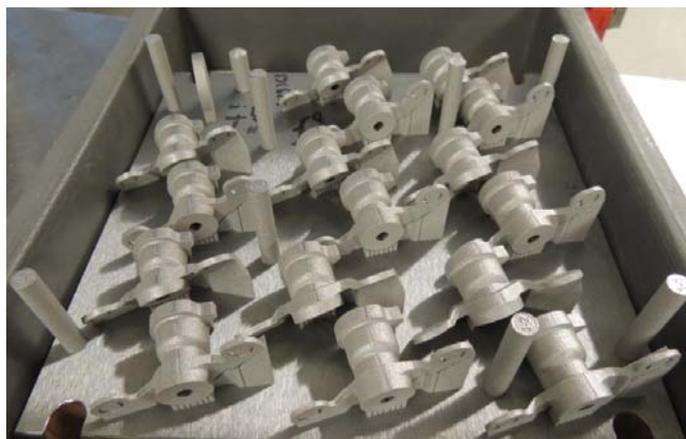
Platform with 16 boroscope bosses and tensile test specimens
