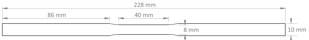
Fig. 1: CMC fatigue specimen geometry
