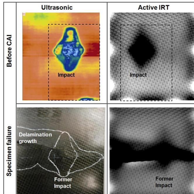
**Fig. 5.** UT and Active IRT results before and after CAI testing (specimen failure).
