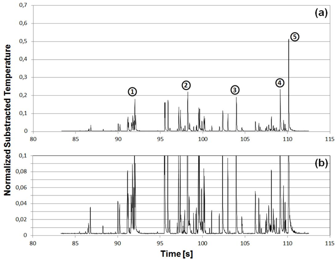
**Fig. 3.** Normalized subtracted temperature (NST)/Timing graph (a) highlighting the 5 main (largest) indications; and (b) magnified low scale NST (from 0 to 0.1) for observation of all recorded peaks related to damage apparition. Note: Normalized subtracted temperature is calculated from raw thermographs by using processing algorithms [3,8].
