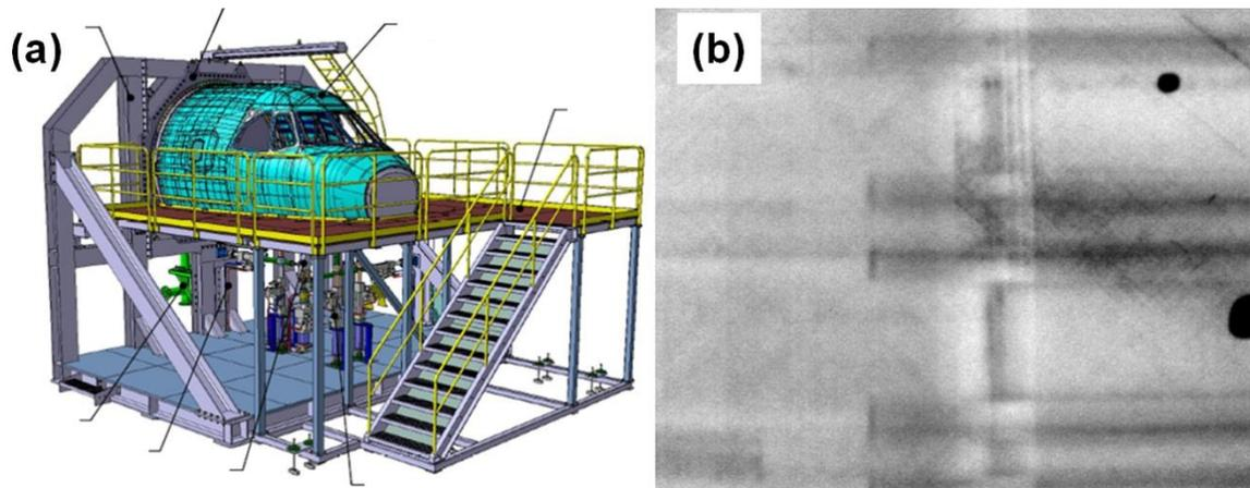
**Fig. 7.** (a) View of testing rig for CFRP cabin; and (b) active thermograph showing structural information and indications related to skin delaminations (black spots).
