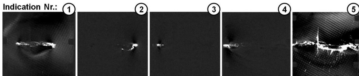
**Fig. 4.** Passive thermographs obtained from main indication (1 to 5) after image processing (Normalized subtracted temperature).
