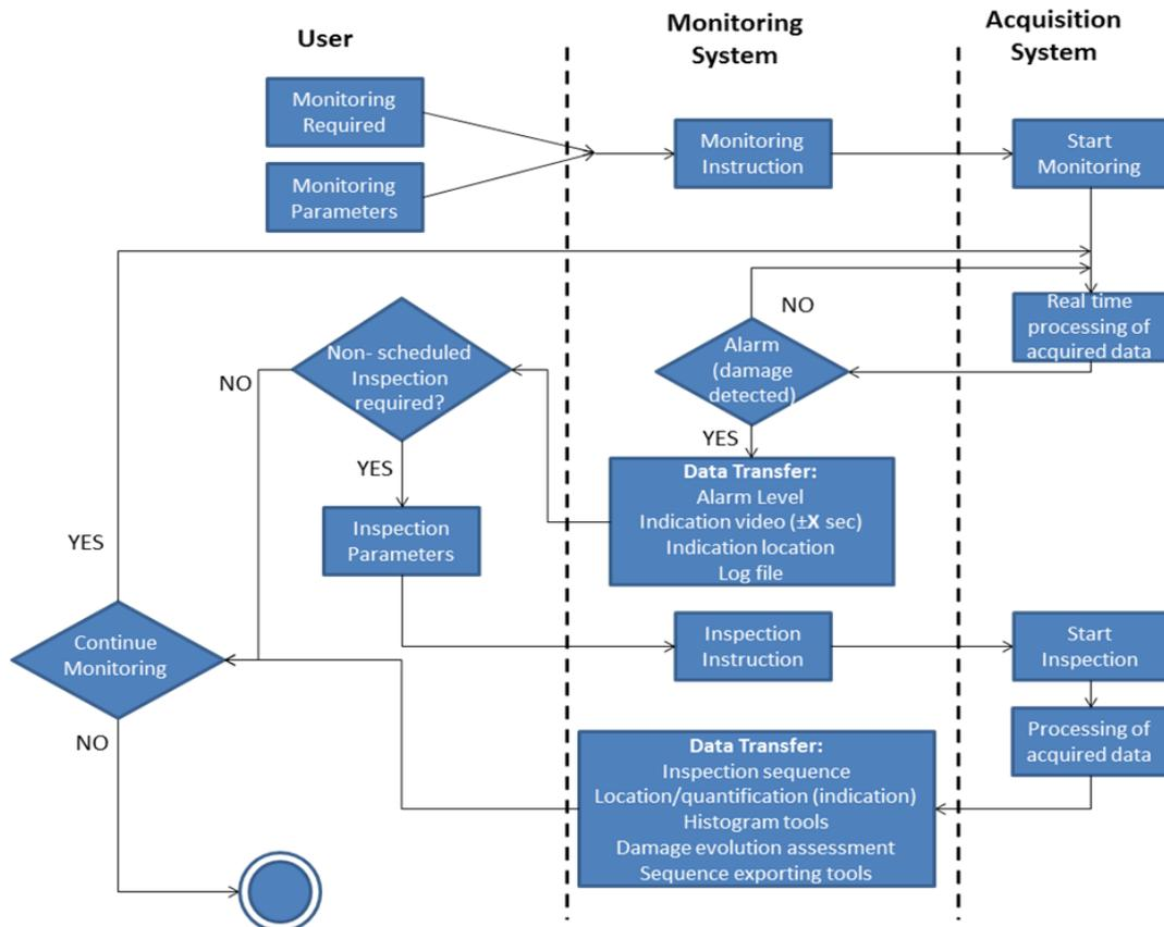
**Fig. 6.** Use case for continuous monitoring.
