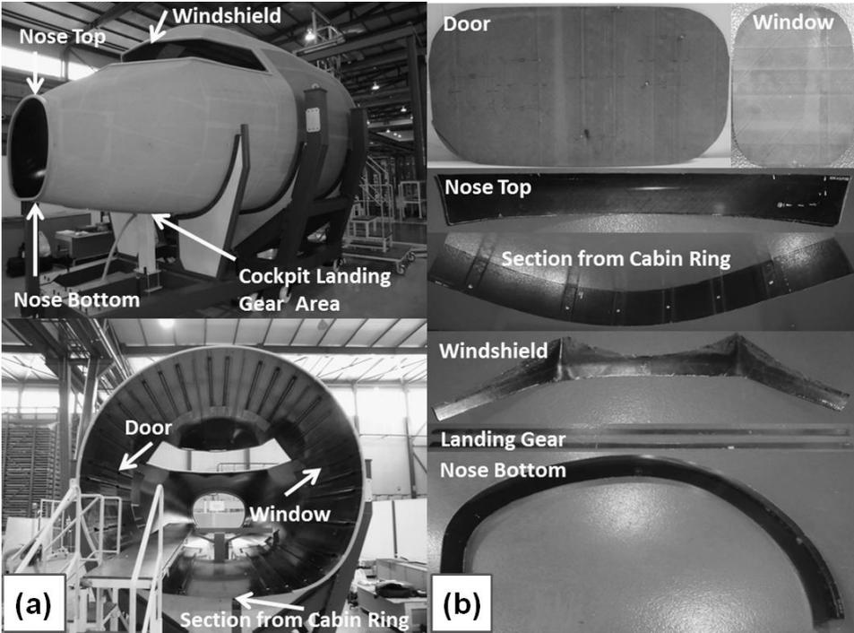
**Fig. 1.** (a) CFRP cockpit views with indication of main area for part preparation; and (b) inspected specimens.
