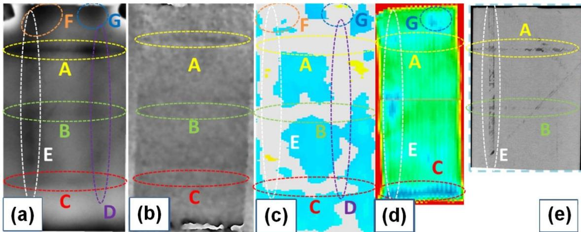
**Fig. 2.** Inspection results for the different NDT methods under evaluation for damage monitoring system: (a) Active thermography; (b) Laser Shearography; (c) Conventional and (d) Air coupled ultrasonics; and (e) Computed tomography cross section for sample evaluation.
