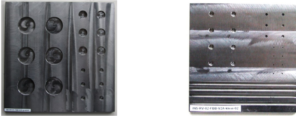
Fig. 1. Backside of the V2A test specimens with sizes of 200 x 200 x 7.5 mm 3 (left) and of 100 x 100 x 4.5 mm 3 (right) with flat bottom holes with different diameters and remaining wall thicknesses.
