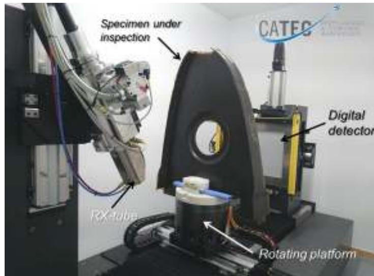
Figure 5. View of computed tomography system at CATEC facilities.
