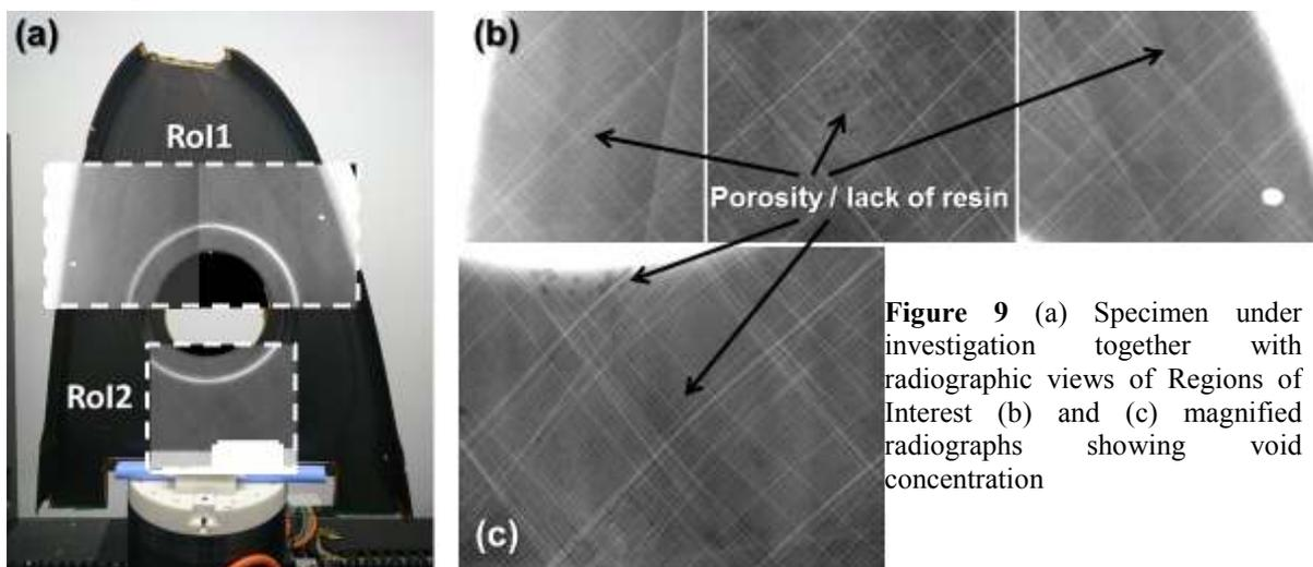
**Figure 9** (a) Specimen under investigation together with radiographic views of Regions of Interest (b) and (c) magnified radiographs showing void concentration
