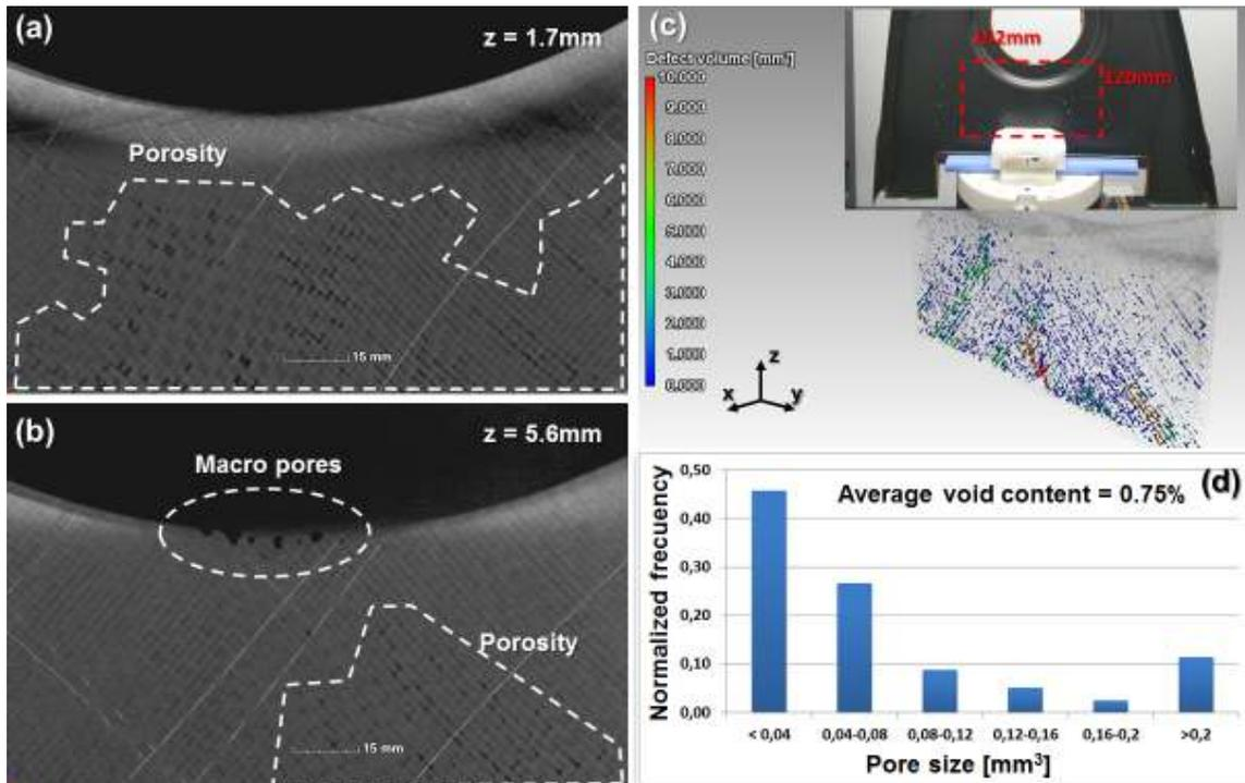
**Figure 10.** Tomographic investigations on target part: cross sections at (a) 1.7 and (b) 5.6mm thickness position with indication of porosity; (c) 3D representation of detected porosity and Region of Interest (RoI); and (d) histogram with pore size distribution.
