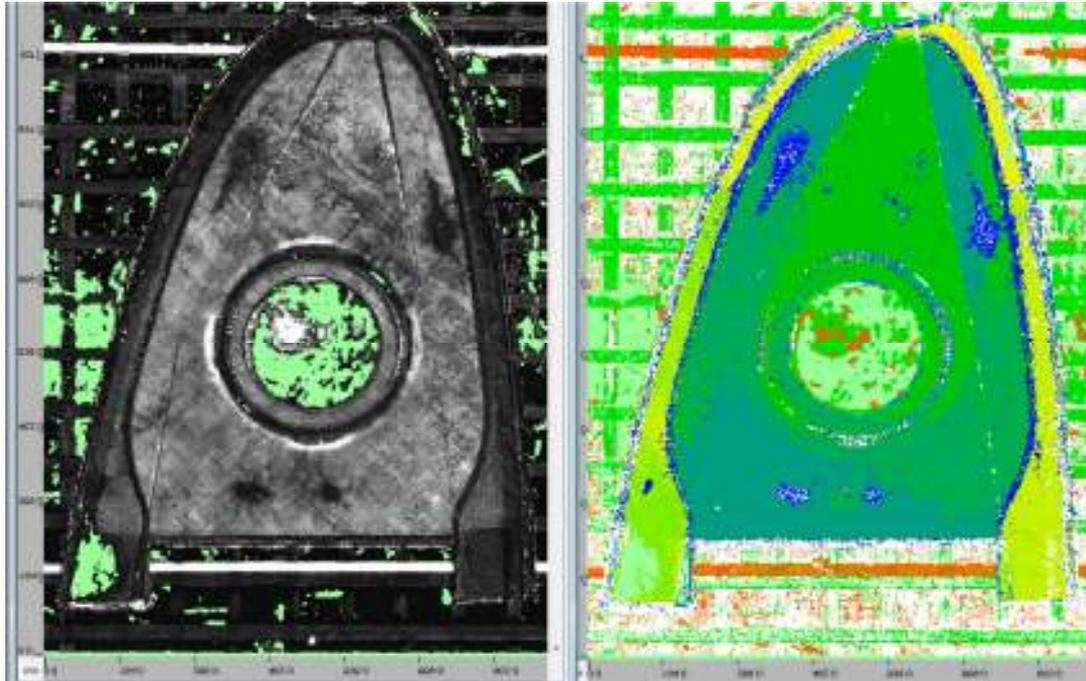
**Figure 8.** tecnaLUS Inspection results of Leading Edge
