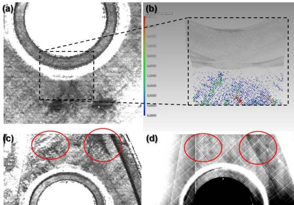
**Figure 11.** Comparison results views from high void content areas: (a) LUT C-Scan and (b) 3D tomographic representation of RoI with void content by 0.75%; (c) LUT C-Scan and (d) Digital radiograph of RoI with porosity accumulation (see red circles). All results shows very good correlation.
