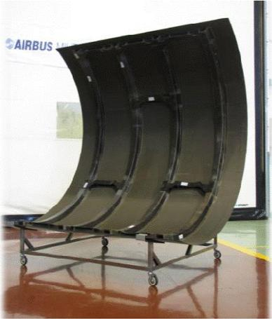
**Figure 1.** Curved panel stiffened by RTM detail parts
